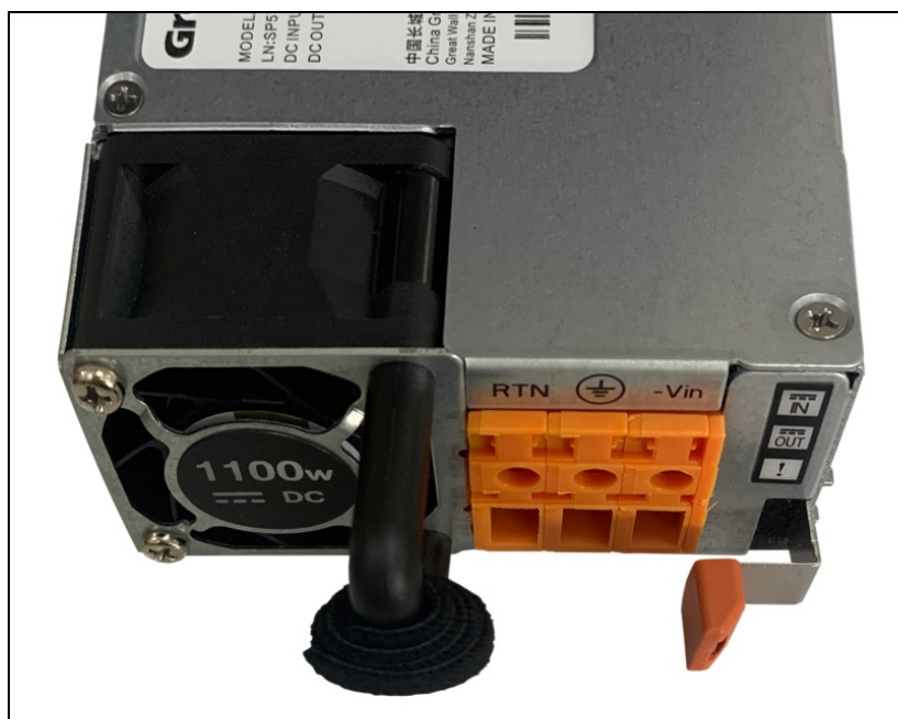
Figure 18. Connector on the ThinkSystem 1100W -48V DC Hot-Swap Gen2 Power Supply
